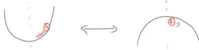
Figure 21: The micromotion is such that when the ion is at its maximal point, it gets pushed back in maximally.
